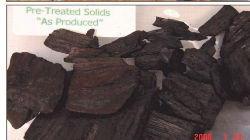
Waste loblolly pine wood (top) and after hydrothermal pretreatment (bottom).
