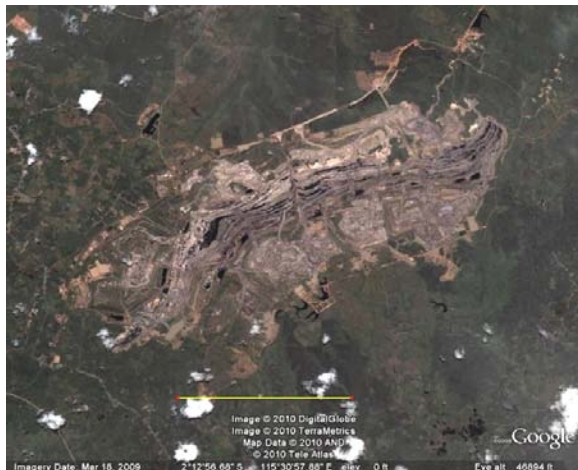
Fig. 3. Closer view image of coal mining area in Fig. 2 showing (black) coal seams dipping gently towards the NNW. Yellow scale bar is ~0.5 km.
